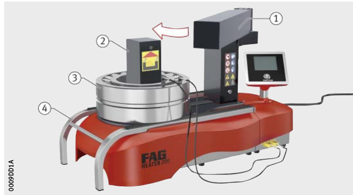
Figure 2 Heating of rolling bearing
