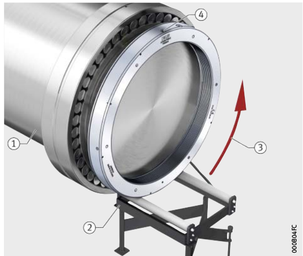
Figure 35 Unscrewing the hydraulic nut
