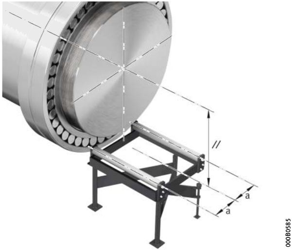
Figure 16 Aligning the mounting aid
