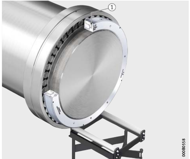
Figure 21 Loosening the hydraulic nut slightly
