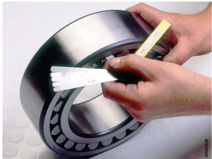
Figure 7 Measurement of radial internal clearance using feeler gauges
