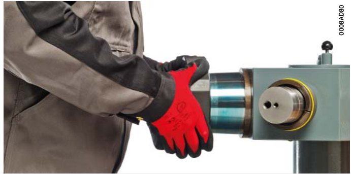
Figure 5 Touching with a taper ring gauge
