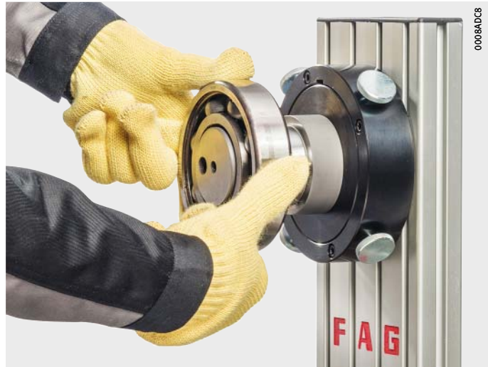
Figure 14 Sliding into place of heated bearing parts
