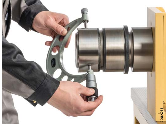
Figure 3 Measurement of expansion using external micrometer
