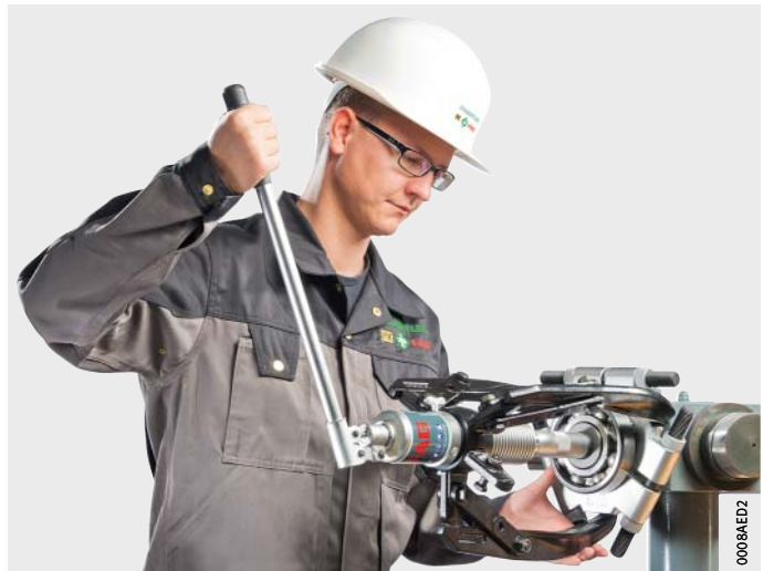
Figure 1 Dismounting by means of extraction device
