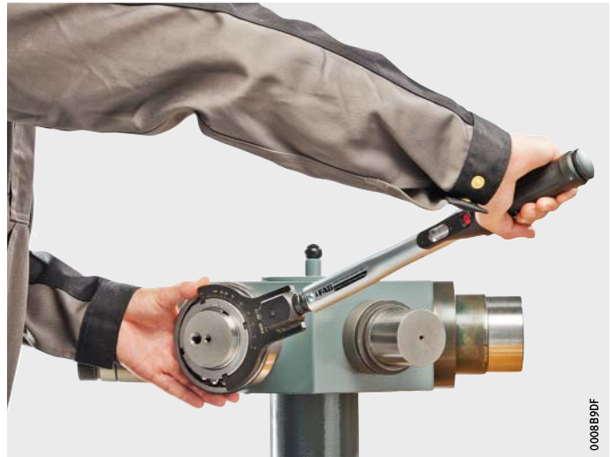
Figure 11 Mounting by means of double hook wrench
