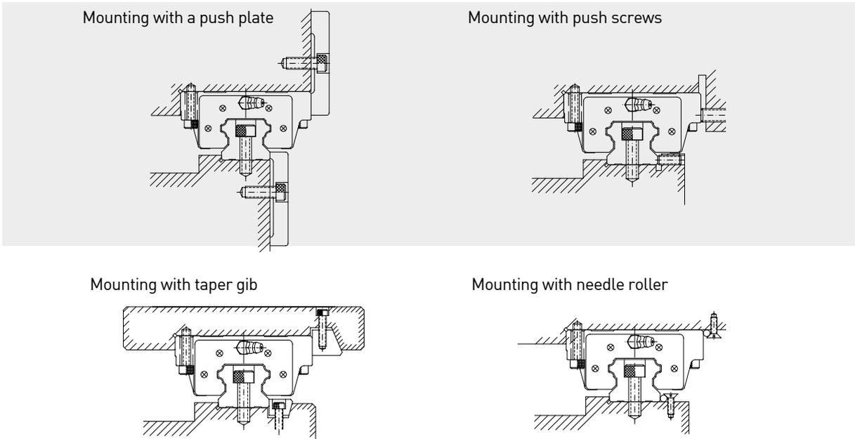
**(2) Procedure of rail installation**
