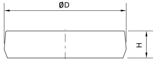
Table 2-7-7 Dimensions of Bolt Caps for Rail Mounting Holes
