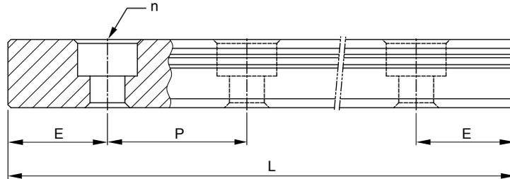
$$L = (n - 1) \times P + 2 \times E \quad \dots \dots \dots \text{Eq.2.4}$$
