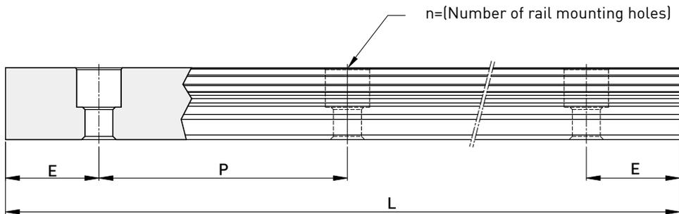
$$L = (n - 1) \times P + 2 \times E \quad \dots \dots \dots \text{Eq.2.2}$$
