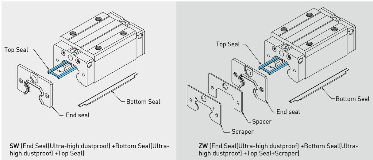
Note : 1. The available size for high dust proof accessories are HG15C, HG20(C/H), HG30(C/H), HG35(C/H), HG45(C/H).
