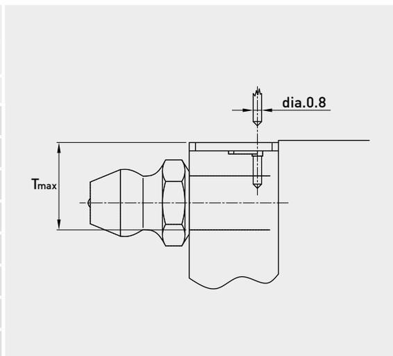
○ The lubricant amount for a block filled with grease
