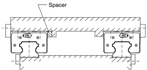
**HGW type block with mounting holes in different directions.**
