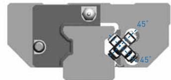
(2) Low Noise Design With SynchMotion™ technology, rolling elements are interposed between the partitions of SynchMotion™ to provide improved circulation. Due to the elimination of contact between the rolling elements, collision noise and sound levels are drastically reduced.
