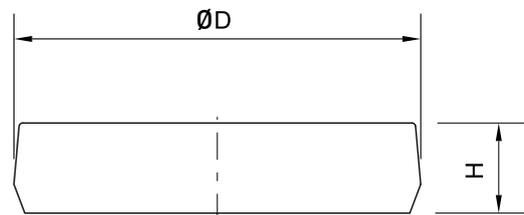
Table 2-2-14 Dimensions of Bolt Caps for Rail Mounting Holes
