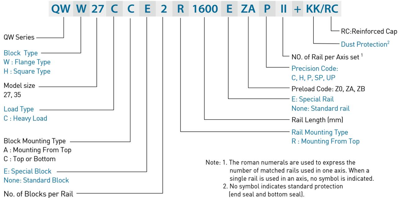
Note: 1. The roman numerals are used to express the number of matched rails used in one axis. When a single rail is used in an axis, no symbol is indicated.
