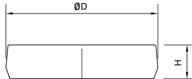
Table 2-8-20 Dimensions of Bolt Caps for Rail Mounting Holes
