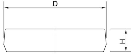
Table 2-1-18 Dimensions of Bolt Caps for Rail Mounting Holes
