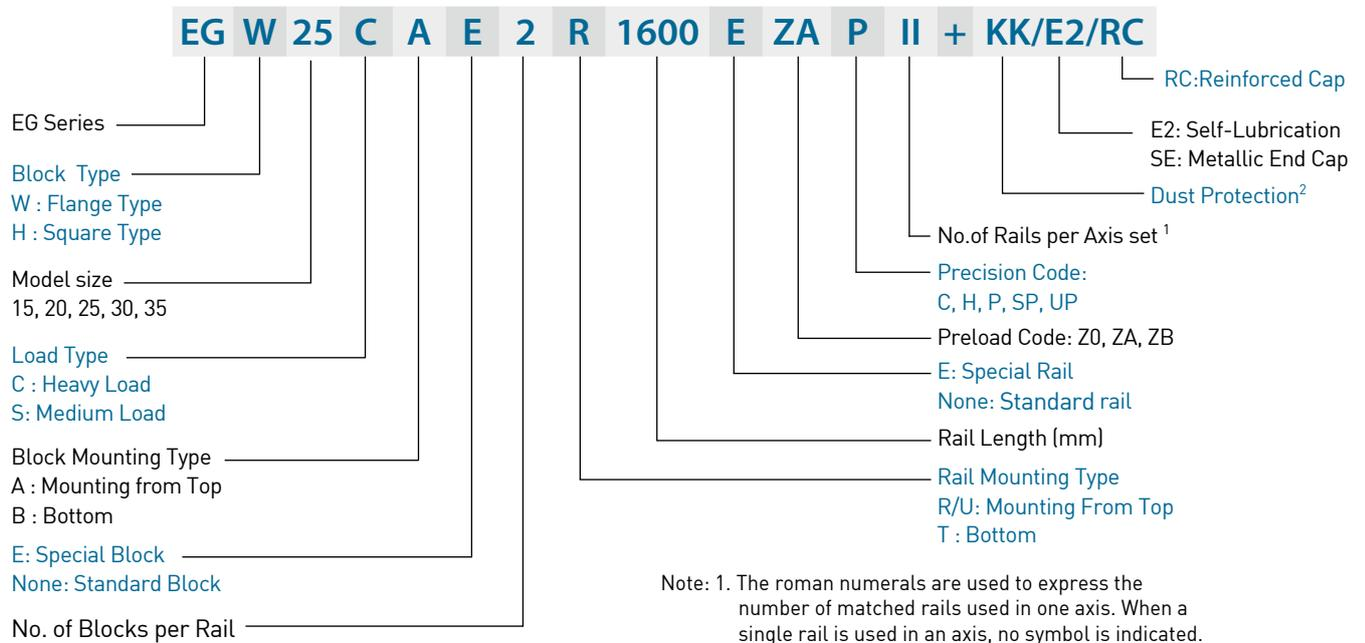
Note: 1. The roman numerals are used to express the number of matched rails used in one axis. When a single rail is used in an axis, no symbol is indicated.
